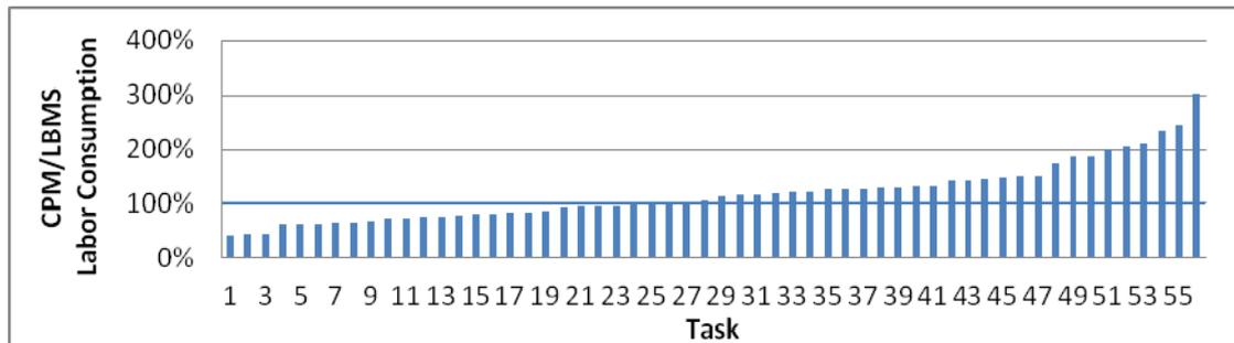
Figure 3: Labor consumption comparison by task. LBMS floor productivity was better for tasks with values greater than 100%.
