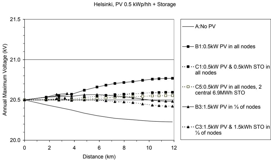
**Figure 4.2:** Annual maximum voltage profiles in Helsinki for cases A, B1, B3, C1, C3, and C5. The installed PV capacity totals 0.5 kW<sub>p</sub> / hh, and the corresponding storage capacity 0.5 kWh / hh.
