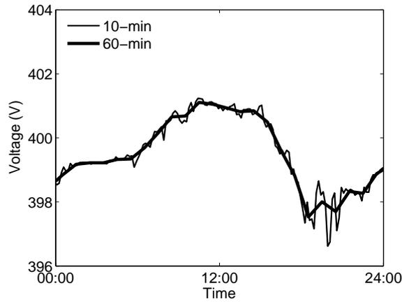
Figure 6: Example of grid voltage during one day at one household node (node 13) with the 1 kW<sub>p</sub> scenario and different averaging times.
