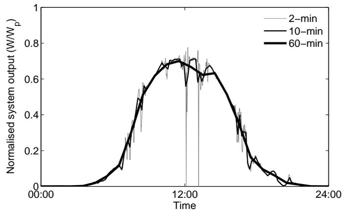
Figure 4: Example of normalised PV system output during one day with different averaging times.
