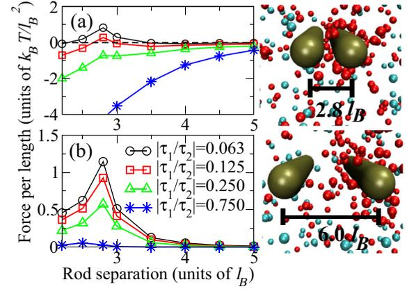
FIG. 1. (a) Total force per length between the rods and (b) osmotic contribution to the force from the cations in the interrod space, for varying rod charge ratio  $|\tau_1/\tau_2|$  and  $\kappa=0.7 l_B^{-1}$ . A positive force corresponds to repulsion. At right, simulation snapshots of the system at two rod separations.
