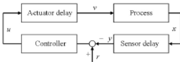
Fig. 1. Control system with network delays
