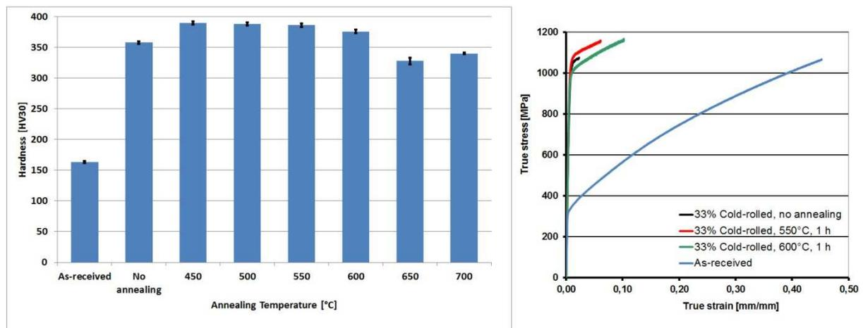
Figure 1. Hardness (left) and tensile behaviour (right) for different thermo-mechanical treatments.
