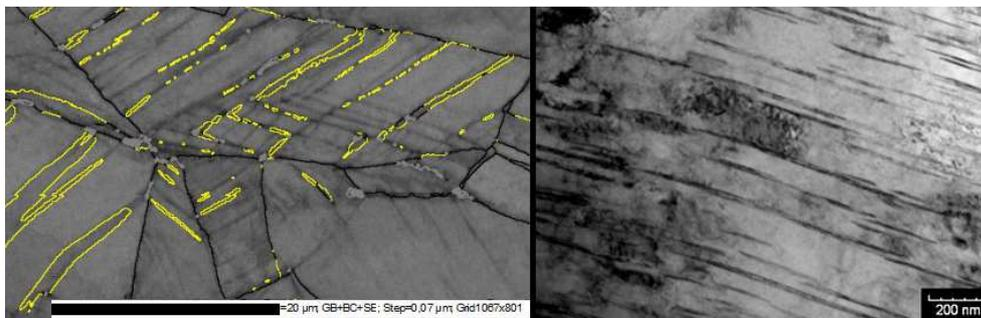
Figure 3. EBSD micrograph of the deformed structure showing twin boundaries in yellow (left) and TEM micrograph (right).
