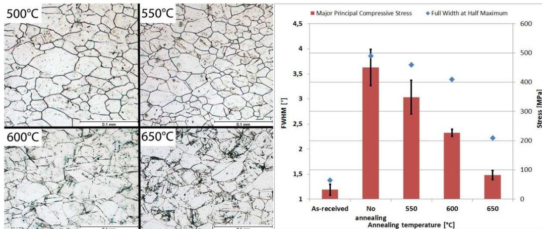
Figure 2. Cold-rolled samples annealed at different temperatures and etched to reveal grain boundaries (left). Residual stress and peak broadening for different treatments (right).
