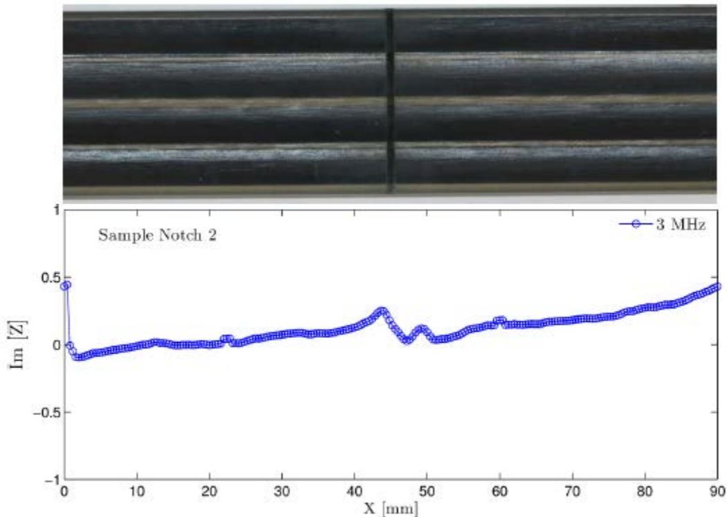
Figure 2. Impedance scan along the length of notched sample
