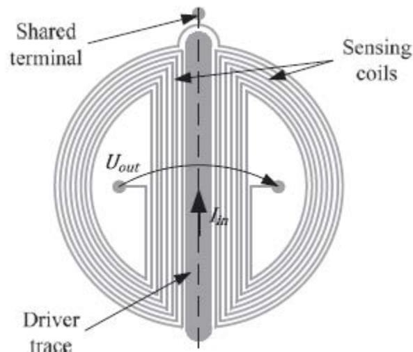
Figure 1. Configuration of the advanced probe [2]
