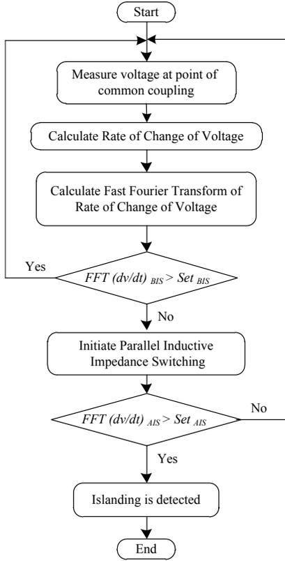
Fig. 9. Flowchart of the proposed islanding detection scheme.
