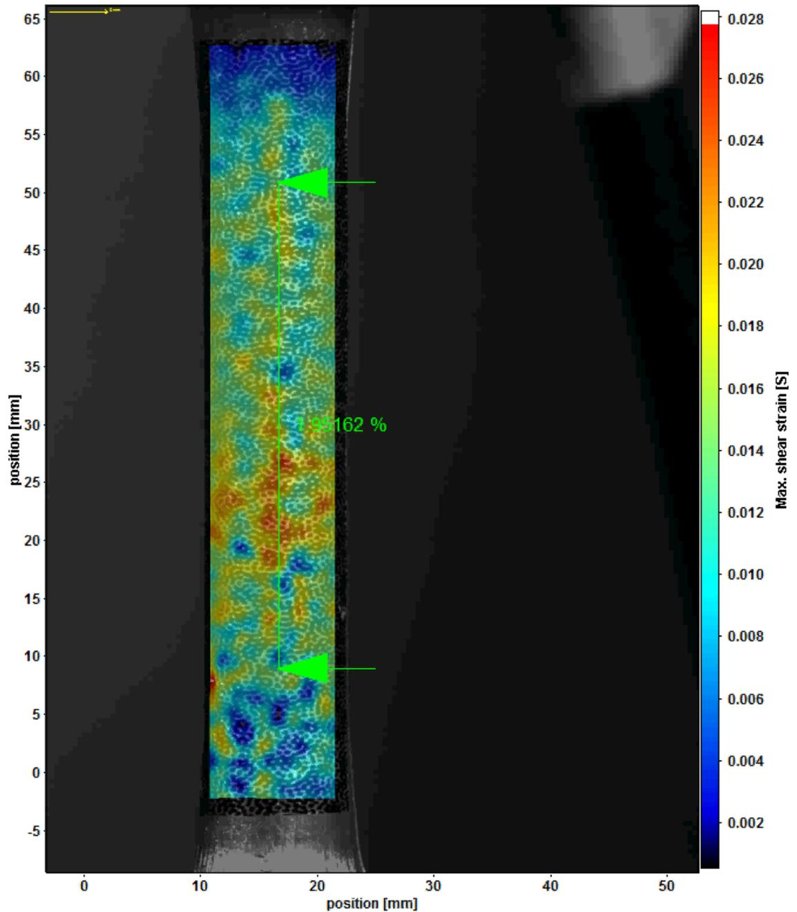
Figure 2: Shear strain fields of A356-T6 at 2% extension.
