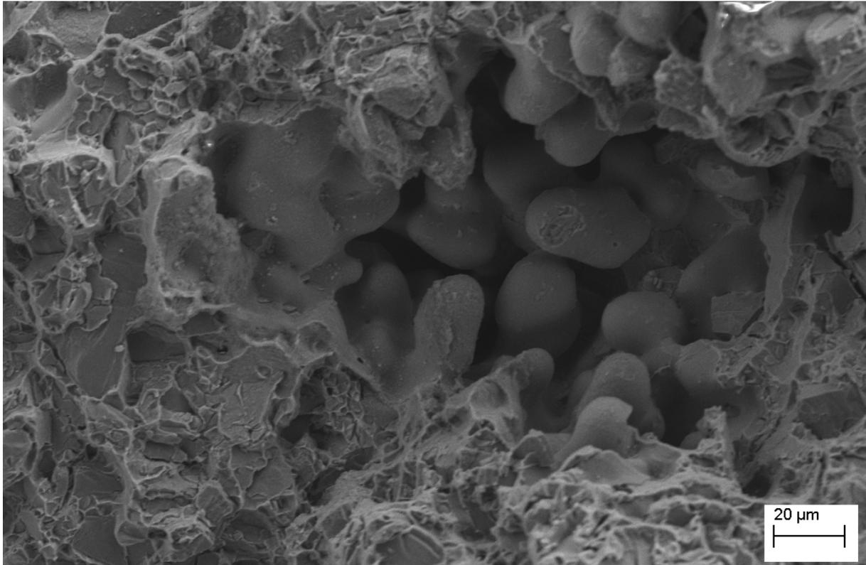
Figure 4: Fractograph of the Al-SiC composite after tensile testing.
