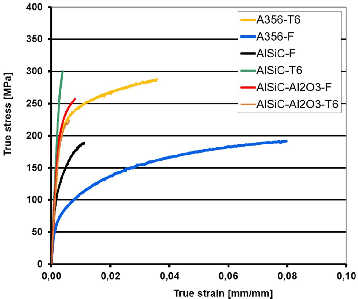
Figure 3: True stress-true strain curves of the tested alloys.
