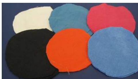
**Figure 1.** Original cotton and dyed cotton fabrics: top line: original cotton, direct blue, direct red; bottom line: reactive black, reactive orange and vat dyed blue
