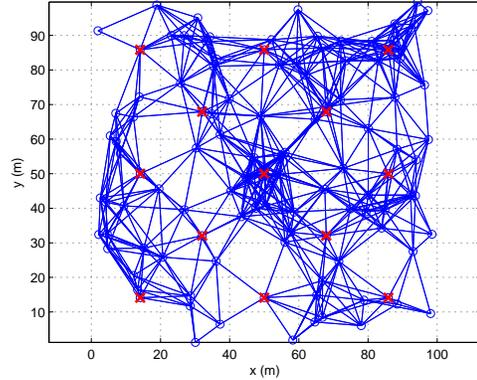
Figure 1: Scenario of the simulations. Red crosses indicate the positions of 13 anchor nodes, blue circles the positions of the other 100 nodes and blue lines the edges of the graph. Communication radius is 20 m.
