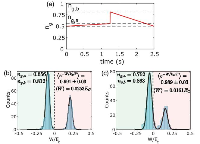
FIG. 3. (a) Protocol used to extract work with high probability (see text). (b),(c) Work histograms and experimental values of work and exponentiated work averages obtained for (b)  $n_{g,a} = 0.656$ ,  $n_{g,b} = 0.698$  and (c)  $n_{g,a} = 0.752$ ,  $n_{g,b} = 0.863$ , with ramp time  $t_1 = 1.25$  s. The vertical dashed line sets the zero free energy difference to guide the eye. Solid lines are obtained by numerically solving the master equation [27].
