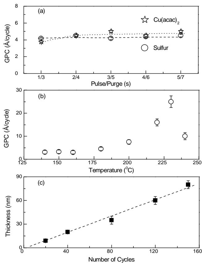
**Figure 1.** Optimization of the deposition parameters: (a) GPC versus precursor pulse lengths, (b) GPC versus deposition temperature, and (c) film thickness versus number of ALD cycles. In (a) and (c), the deposition temperature was 160 °C. Note that in (a) the purge time was increased together with increasing precursor pulse time such that the purge time was always longer than the precursor pulse time to ensure the complete removal of the precursor excess and the reaction by-products.
