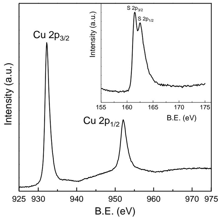
**Figure 5.** High-resolution XPS spectra for a copper sulfide thin film deposited at 150 °C, recorded after sputtering the film surface with Ar for 30 s.
