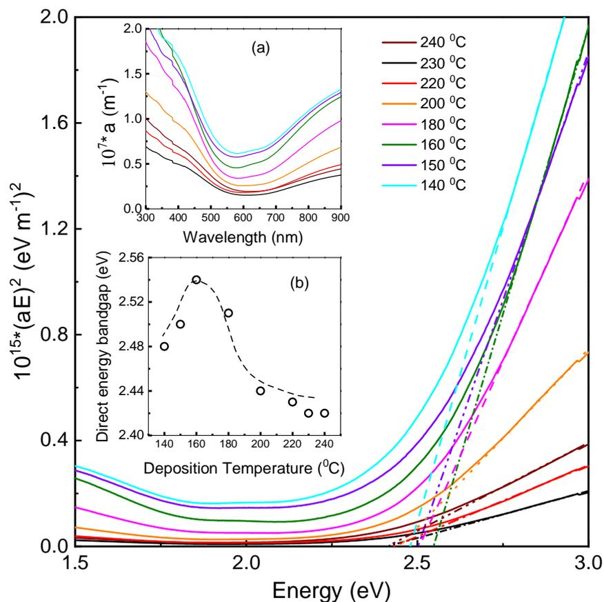
**Figure 6.** Tauc plots for the determination of the direct bandgap for the copper sulfide thin films deposited at different temperatures. In each case the extrapolated interception of the linear portion of the curve with the energy axis gives the optical bandgap of the film. Inset (a) displays the absorption coefficient of the films as a function of wavelength. Inset (b) shows the dependence of the bandgap on the deposition temperature; the dotted curves are for a guide to the eyes.
