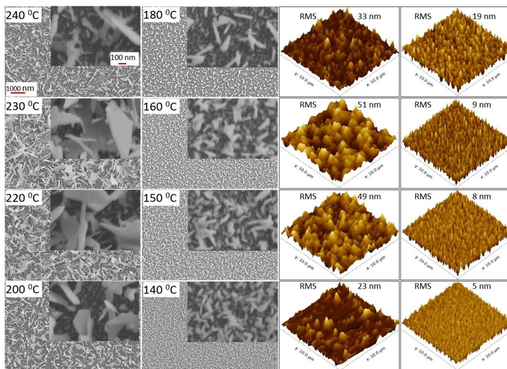
**Figure 4.** SEM (left) and AFM (right) images for the copper sulfide thin films deposited at different temperatures.
