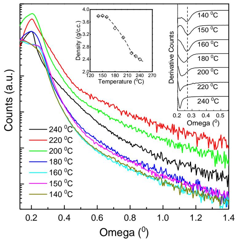
**Figure 3.** XRR patterns for the copper sulfide thin films deposited at different temperatures; derivative plots in the inset.
