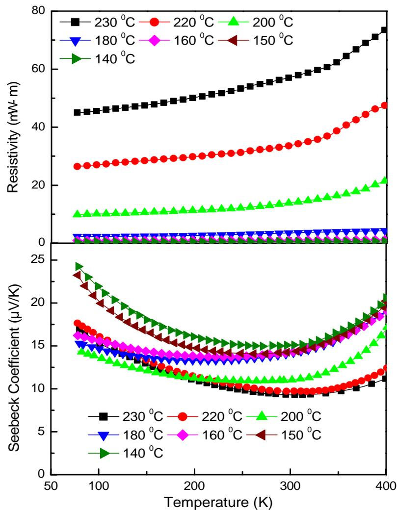
**Figure 7.** Electrical resistivity and Seebeck coefficient of the copper sulfide thin films deposited at different temperatures.
