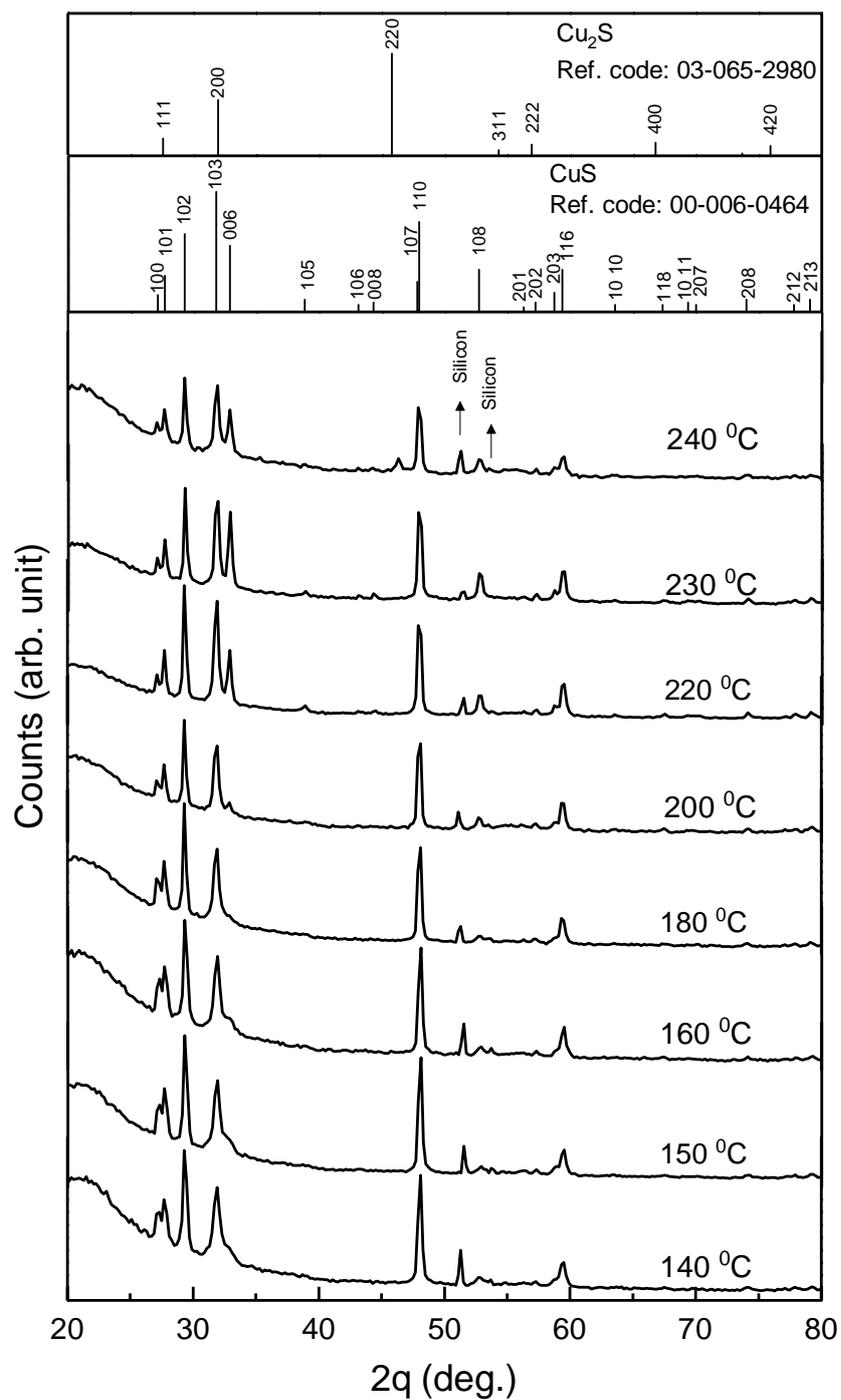
**Figure 2.** XRD patterns for the copper sulfide thin films deposited at different temperatures.
