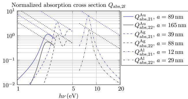
FIG. 4. Normalized dipole and quadrupole absorption cross sections  $Q_{abs,2l}^{Ax}$ ,  $l = 1, 2$ , for a sphere made of gold (Au), silver (Ag), and aluminum (Al), and where the radius  $a$  has been tuned to match the condition (60) for optimal absorption; see also Fig. 3. The almost tangent optimal bounds are plotted as dotted lines. Here, the background is lossless with  $\epsilon_b = 1$ .
