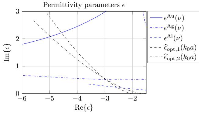
FIG. 3. The dielectric functions  $\epsilon^{Ax}(\nu)$  for gold (Au), silver (Ag), and aluminum (Al) according to the Brendel-Bormann model [26], and the asymptotic near-optimal dielectric functions  $\hat{\epsilon}_{opt,l}(k_0a)$ ,  $l = 1, 2$ , parametrized by frequency  $\nu$  and electrical size  $k_0a$ , respectively, plotted in the complex plane. Their intersections give an approximation to an optimal dipole or quadrupole resonance for each metal.
