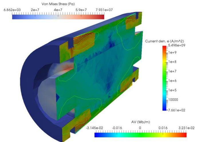
Fig. 1. Von Mises stress (rotor surface), elementary current density (slice) and magnetic vector potential (contour) of the damaged rotor after the simulation (50 ms). The increase of current density on the hot spot is shown in the upper part of the forward end ring.
