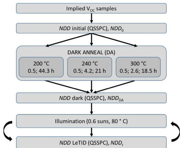
**Fig. 1.** Process sequence of the studied implied  $V_{oc}$  samples. The NDD was continuously measured during the illumination time. The reference sample (*i.e.* no DA after firing) is not included in the figure.
