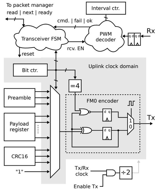
Fig. 7. Transceiver structure
