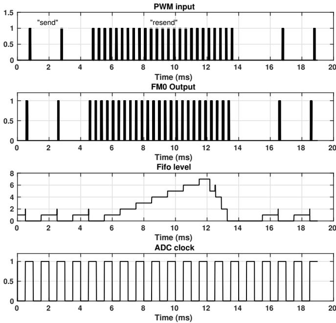
Fig. 11. Simulation of data loss and retransmission.
