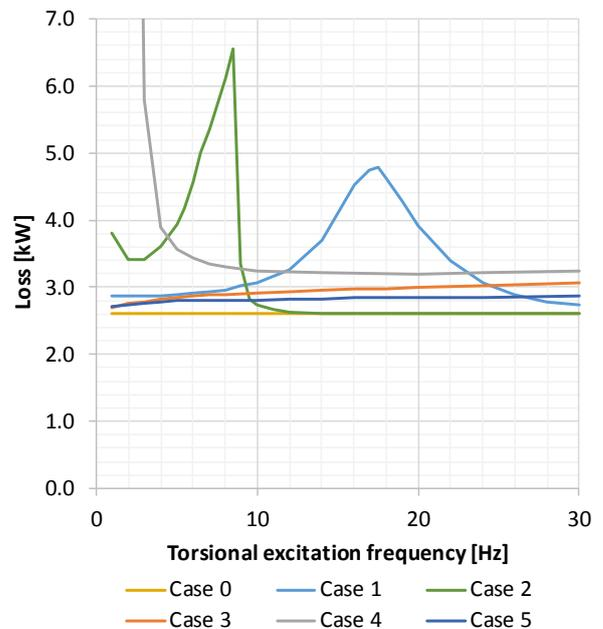
Fig. 1. Total electromagnetic loss of the 37 kW motor as a function of excitation frequency under different control modes of the harmonics. Cases 0 ... 5 are defined in the main text.
