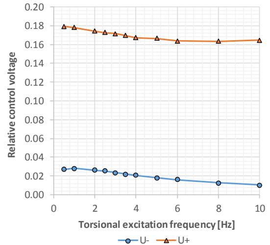
Fig. 12. Amplitudes of voltage harmonics needed to suppress the torsional vibration and lower current harmonic of the 6 MW motor (Case 3).
