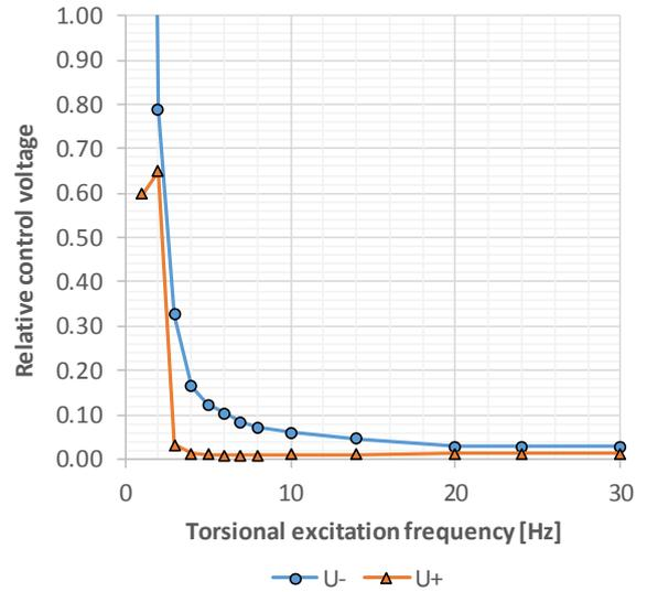
Fig. 6. Amplitudes of voltage harmonics needed to suppress the torsional vibration and upper current harmonic of the 37 kW motor (Case 4).
