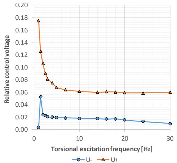
Fig. 7. Amplitudes of voltage harmonics that suppress the torsional vibration and give the minimum electromagnetic loss for the 37 kW motor (Case 5).
