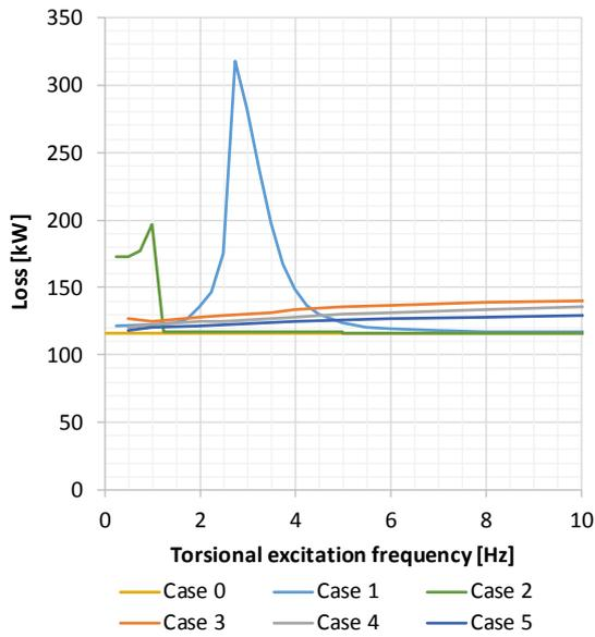
Fig. 8. Total electromagnetic loss of the 6 MW synchronous motor as a function of excitation frequency under different control modes of harmonics. The Cases are defined on the second page of this text.
