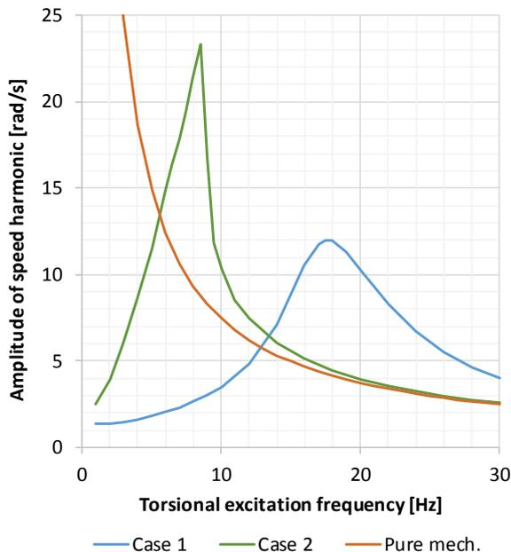
Fig. 2. Amplitudes of vibration harmonic in the rotation speed of the 37 kW motor for Cases 1 and 2. The third curve presents the amplitude obtained from the equation of motion when neglecting the electromagnetic effects.
