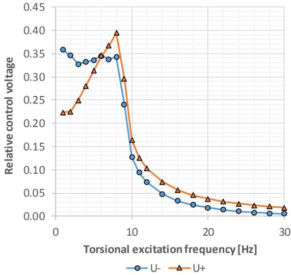
Fig. 4. Amplitudes of voltage harmonics needed to suppress the first-order vibration harmonics from the stator current of the 37 kW motor (Case 2).
