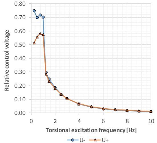
Fig. 11. Amplitudes of voltage harmonics needed to suppress the first-order vibration harmonics from the stator current of the 6 MW motor (Case 2).
