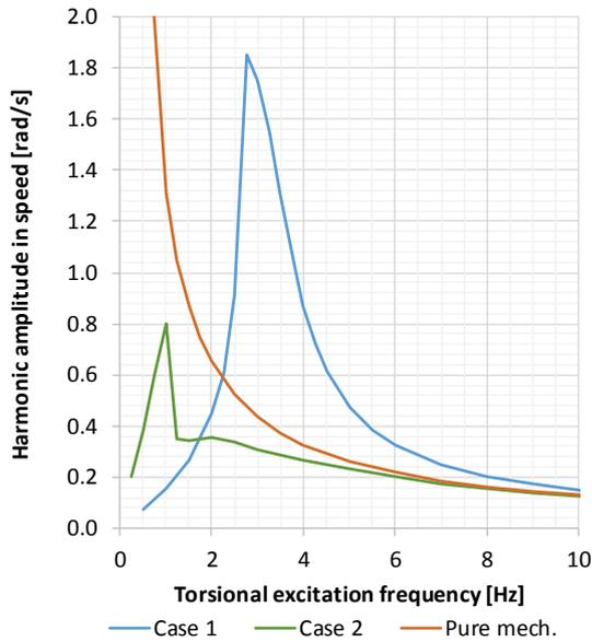
Fig. 9. Amplitudes of vibration harmonic in the rotation speed of the 6 MW motor for Cases 1 and 2. The third curve presents the amplitude obtained from the equation of motion when neglecting the electromagnetic effects.
