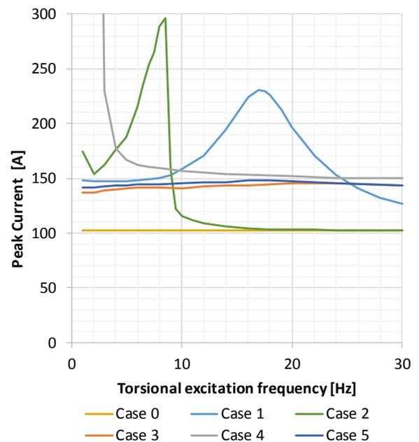
Fig. 3. Peak values of the terminal currents of the 37 kW motor for the different Cases studied.
