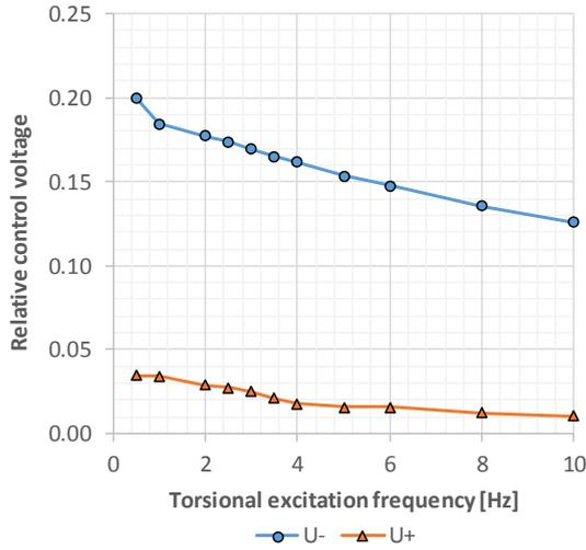
Fig. 13. Amplitudes of voltage harmonics needed to suppress the torsional vibration and upper current harmonic of the 6 MW motor (Case 4).
