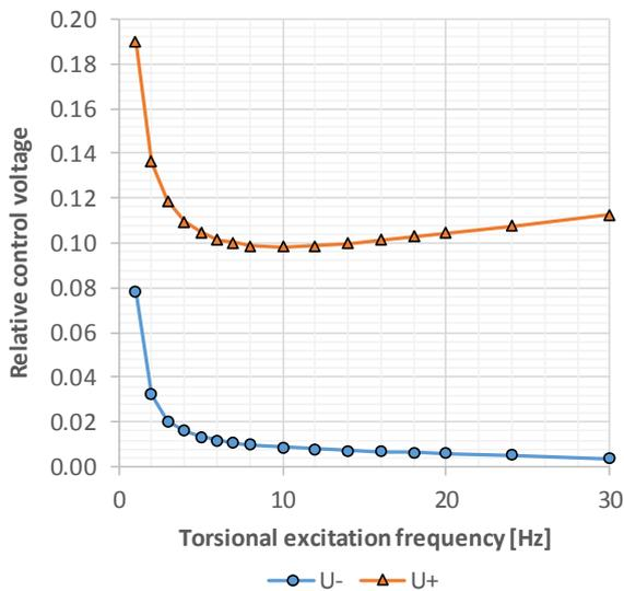
Fig. 5. Amplitudes of voltage harmonics needed to suppress the torsional vibration and lower current harmonic of the 37 kW motor (Case 3).
