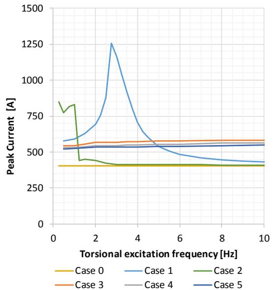
Fig. 10. Peak values of terminal currents of the 6 MW motor for the different Cases studied.
