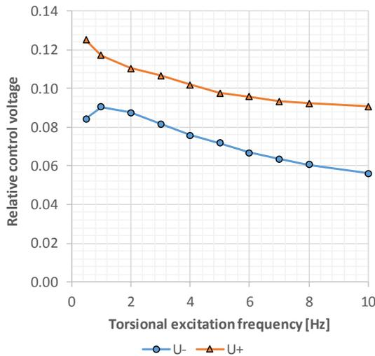
Fig. 14. Amplitudes of voltage harmonics that suppress the torsional vibration and lead to the minimum electromagnetic loss of the 6 MW motor (Case 5).
