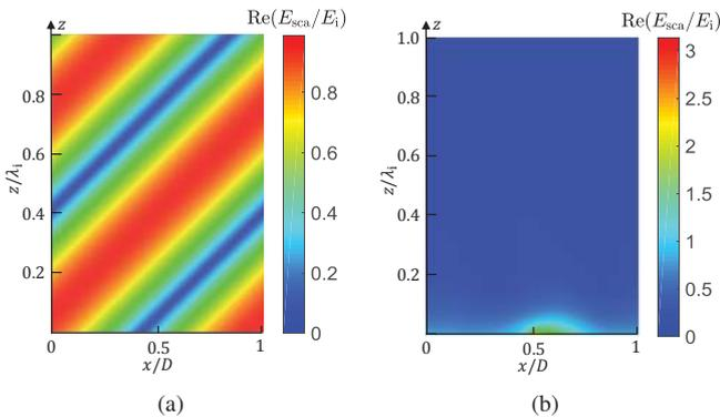
Fig. 4. Instantaneous values of the scattered electric field when incident from (a)  $\theta_i = 45^\circ$  and (b)  $\theta_i = -45^\circ$ . The field value is normalized with the incident field amplitude. The surface impedance is defined for  $R_1 = 0.99$ .
