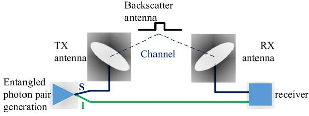
Fig. 1. An illustration of bistatic QI-enhanced QBC systems.
