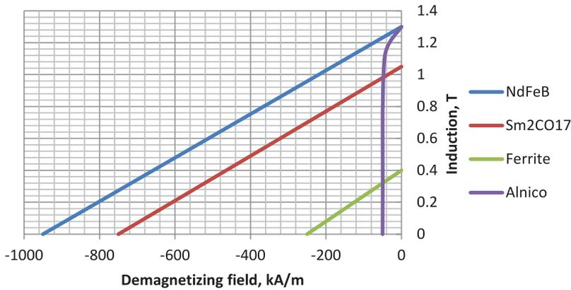
Fig. 1. Demagnetization curves for different permanent magnet materials.
