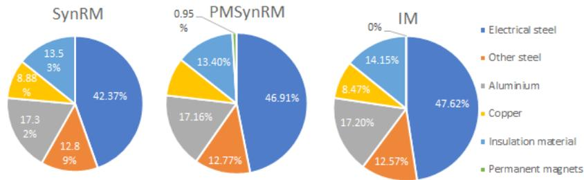
Fig. 2. Percentage ratio of raw materials used for production of different 10kW motors.
