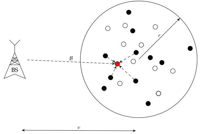
Fig. 1: D2D caching cluster system model example when the cluster is a disk of radius  $r$ . Instead of always having to contact a remote base station (BS), users in the cluster are able to communicate with each other through direct links. The cost of using the traditional downlink is  $B$ . The distance between the BS and the center of the cluster is  $v$ .
