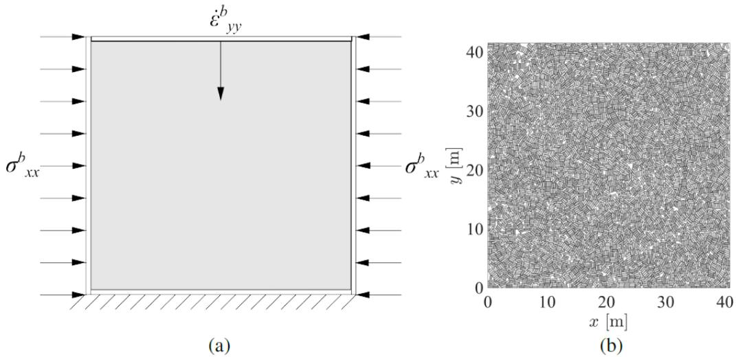
Figure 1. Virtual compression experiments: (a) simulation set-up and (b) a 5000 block sample in its initial configuration. The confining stress  $\sigma_{xx}^b$  was kept equal to 5 kPa and the cover moved down at the constant strain rate of  $5 \times 10^{-4} s^{-1}$ .
