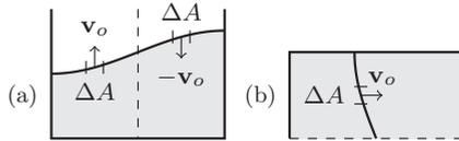
FIG. 1. Alternative formulation of a standing surface wave (a), where the two halves can be redrawn with a common impervious interface (b) moving at velocity  $\mathbf{v}_o$ .
