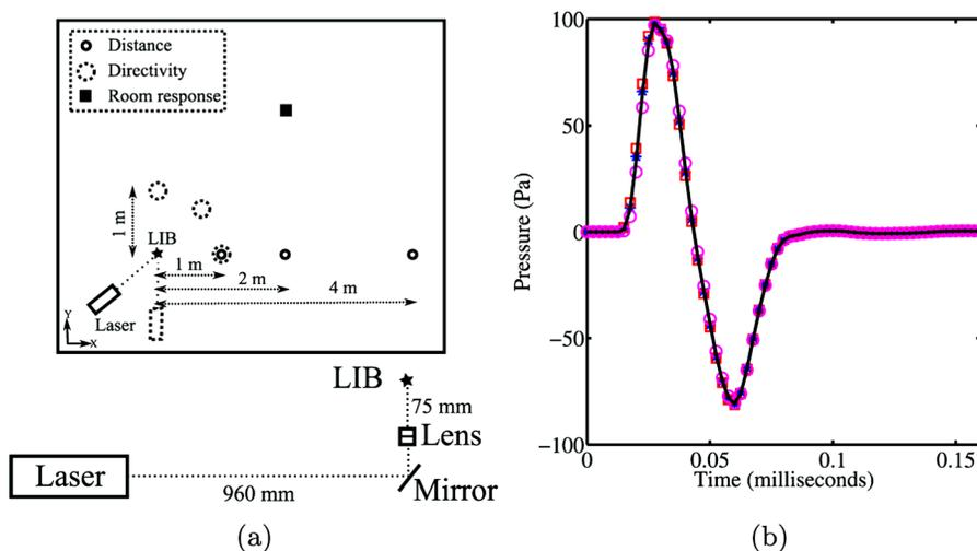
Fig. 1. (Color online) (a) Measurements setup. (b) Averaged pressure pulse wave-forms of three sets of 30 measurements (circles, squares, and stars, respectively) and the average of 100 measurements (solid line).
