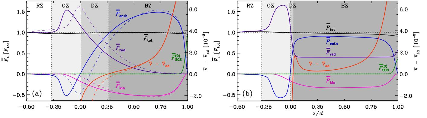
**Figure 1.** Solid lines: radiative (purple), enthalpy (blue), kinetic energy (magenta), and SGS (green) fluxes for Runs K (a) and S (b). Red:  $\nabla - \nabla_{\text{ad}}$ . Dashed lines in (a): corresponding data from Run P. The thick horizontal lines on the abscissae mark the extent of the MZ.
