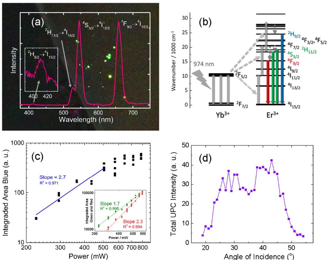
Figure 3. (a) Upconversion emission spectrum for a representative (Y,Yb,Er)-pyrazine thin film grown on Si substrate. The background shows a composite image of the film excited at 974 nm in different spots (taken through a NIR blocking filter). (b) A schematic presentation of the up-conversion mechanism. (c) Laser pump power dependencies for the (Y,Yb,Er)-pyrazine thin film, and (d) dependence of the UPC emission intensity on the incident angle of excitation.
