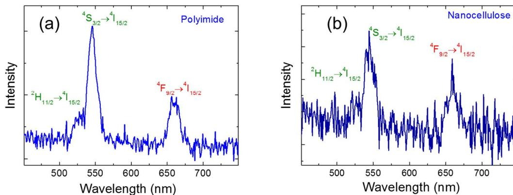
Figure 4. Upconversion emission spectra for (Y,Yb,Er)-pyrazine thin films deposited on flexible (a) polyimide and (b) nanocellulose substrates.
