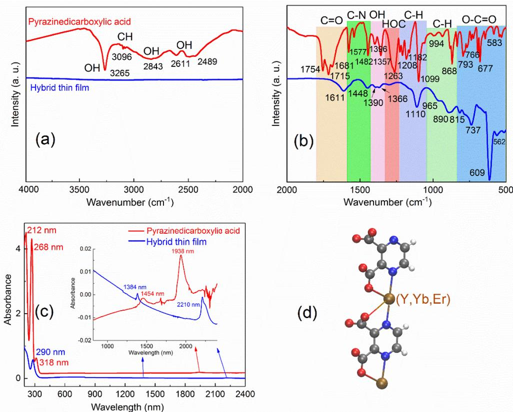
Figure 2. (a,b) FTIR spectra for our hybrid (Y,Yb,Er)-pyrazine thin film and the pyrazine-2,3-carboxylic acid precursor, and (c) UV-vis-NIR-absorption spectrum for the same (Y,Yb,Er)-pyrazine thin-film sample. (d) Possible bonding scheme based on the FTIR data.
