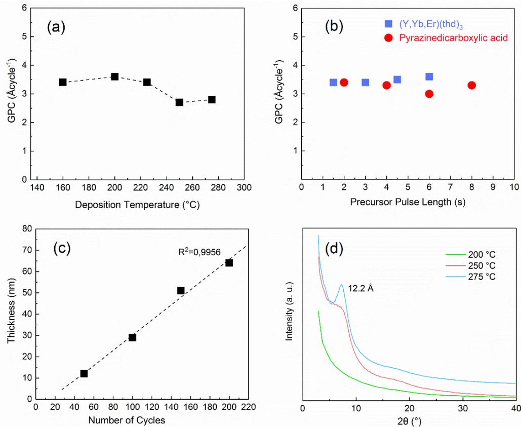
Figure 1. Optimization of the ALD/MLD film growth parameters: (a) growth-per-cycle (GPC) as a function of deposition temperature (150 ALD/MLD cycles) (b) GPC as a function of precursor pulse lengths (deposition temperature 160 °C, 150 ALD/MLD cycles), and (c) film thickness as a function of the number of ALD/MLD cycles (deposition temperature 160 °C). (d) GIXRD patterns for thin films grown at 200-275 °C.
