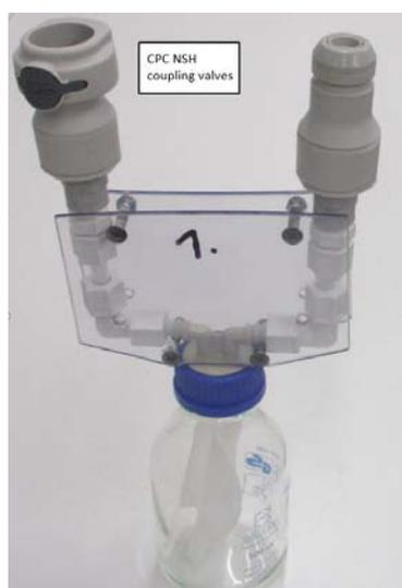
**Fig. 4.** The sample reactor. Duran pressure plus bottles (0.25 dm<sup>3</sup>, 0.5 dm<sup>3</sup> and 1.0 dm<sup>3</sup>) were used as reaction bottles.
