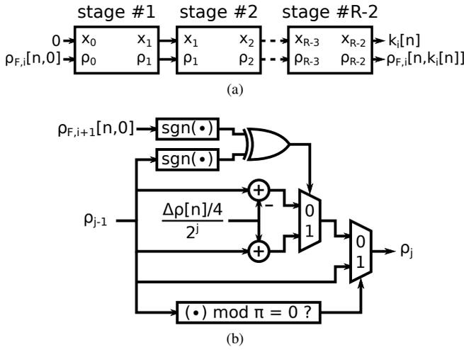
Fig. 6. Datapath that calculates the  $k_i[n]$  output within each DSP engine. (a) Overview of the structure, showing the initial conditions followed by a cascade of  $R - 2$  stages. (b) Implementation of the  $\rho_j$  path inside the  $j$ -th stage (the  $x_j$  path is implemented in a similar fashion).
