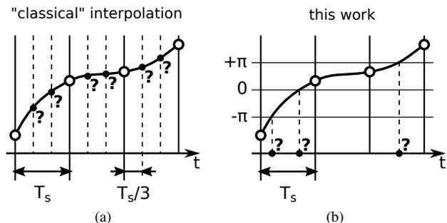
Fig. 2. (a) In “classical” interpolation, the new time instants are known (e.g. multiples of  $T_s/3$ ) and the values of the original function at such time instants are estimated. (b) The DSP of this brief implements the inverse problem: the values are known (e.g. 0,  $\pm\pi$ ), and the time instants at which the original function crosses such values are estimated.
