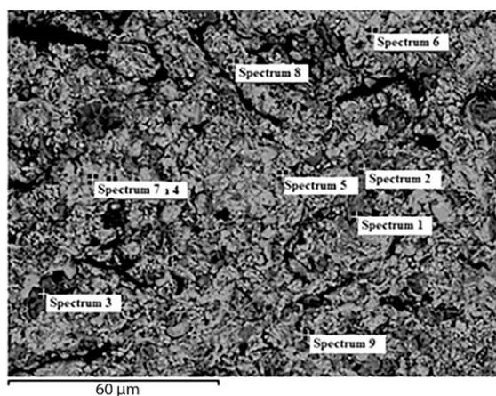
Fig. 3. SEM-EDS analysis for leached residue after Exp. 16
