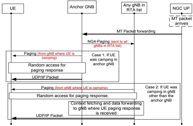
**Figure 3: Potential RAN initiated paging procedure in RRC Inactive.**
