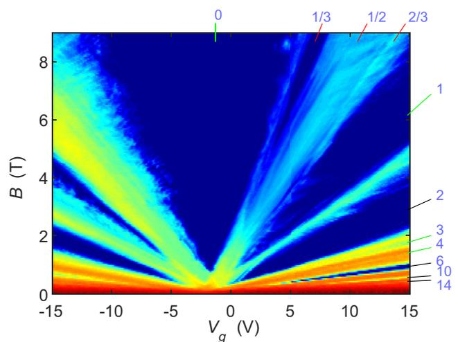
FIG. 2. The magnetoconductance of sample EV2 displayed as a Landau fan diagram on the  $B$  vs gate voltage  $V_g$  plane; data measured at  $f = 3.333$  Hz using ac peak-to-peak excitation current  $I_{p-p} = 0.1$  nA at 20 mK. The region of half filling is given by the slope 0.64 T/V starting from the zero-field Dirac point at  $V_g = -2.3$  V.
