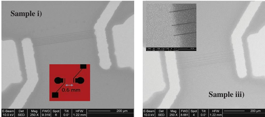
Fig. 1. (a) Line patterns from electron beam exposure of YBCO for sample i), the insert shows a schematic of the electrode layout for four-point-probe measurements. (b) Line patterns for sample iii). The insert shows the region where lines overlapped with the electrical contact.
