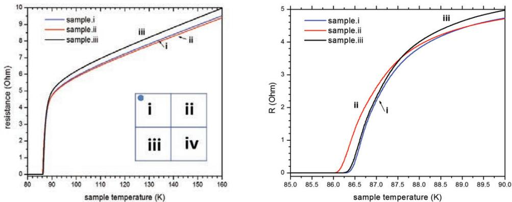
Figure 2. (left) Sample resistances as a function of temperature, (right), sample resistances as a function of temperature around the transition temperature of 86 K.
