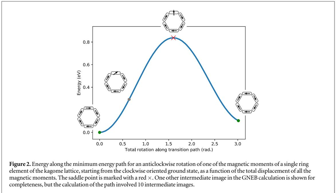
**Figure 2.** Energy along the minimum energy path for an anticlockwise rotation of one of the magnetic moments of a single ring element of the kagome lattice, starting from the clockwise oriented ground state, as a function of the total displacement of all the magnetic moments. The saddle point is marked with a red  $\times$ . One other intermediate image in the GNEB calculation is shown for completeness, but the calculation of the path involved 10 intermediate images.
