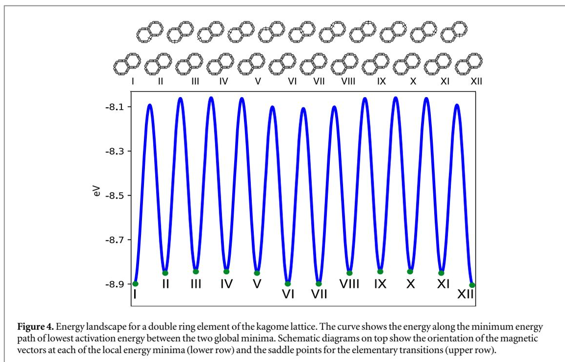
**Figure 4.** Energy landscape for a double ring element of the kagome lattice. The curve shows the energy along the minimum energy path of lowest activation energy between the two global minima. Schematic diagrams on top show the orientation of the magnetic vectors at each of the local energy minima (lower row) and the saddle points for the elementary transitions (upper row).
