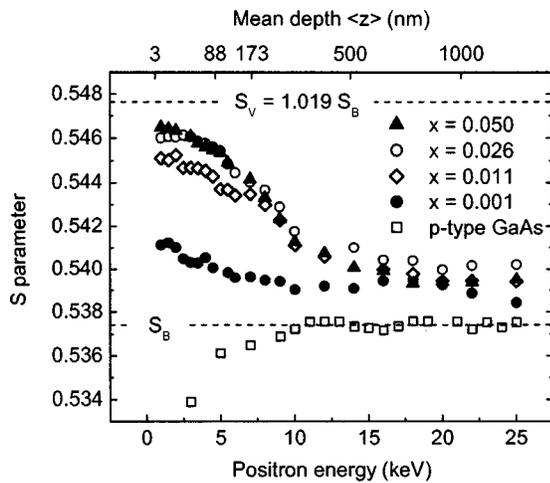
FIG. 1. Low-momentum parameter  $S$  as a function of positron incident energy in the as-grown  $\text{GaAs}_{1-x}\text{N}_x$  samples. The reference value  $S_B$  of  $p$ -type GaAs and the characteristic value  $S_V$  of the  $V_{\text{Ga}}$  are drawn by dashed lines. The top axis shows the mean depth of positron penetration corresponding to the positron incident energy.
