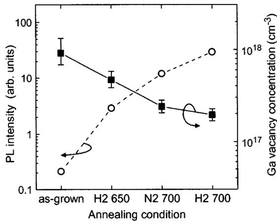
FIG. 5. Integrated PL intensity at 10 K and  $V_{\text{Ga}}$  concentration of 170-nm-thick  $\text{GaAs}_{0.975}\text{N}_{0.025}$  epilayers annealed at different conditions. The lines are guides to the eye.
