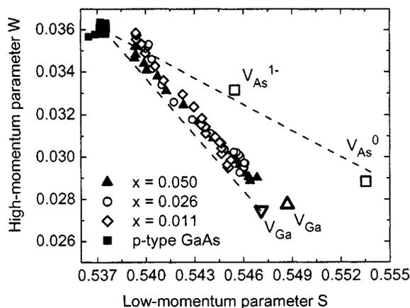
FIG. 2. High-momentum parameter  $W$  as a function of low-momentum parameter  $S$  for as-grown  $\text{GaAs}_{1-x}\text{N}_x$  samples. Characteristic  $W$  and  $S$  parameters for  $V_{\text{As}}$  ( $\square$ ) and  $V_{\text{Ga}}$  ( $\triangle$ ) are from Refs. 18 and 22, respectively, and parameters for  $V_{\text{Ga}}$  ( $\nabla$ ) are measured in this work. The dashed lines are guides for the eye.
