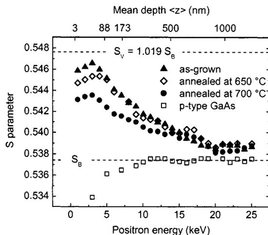
FIG. 4. Low-momentum parameter  $S$  as a function of positron incident energy in  $\text{GaAs}_{0.975}\text{N}_{0.025}$  samples annealed at different temperatures. Other features are identical with Fig. 1.
