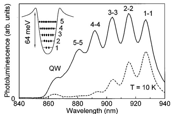
FIG. 1. Low-temperature photoluminescence spectra of the  $\text{In}_x\text{Ga}_{1-x}\text{As}$  quantum dot sample for low (dashed line) and high (solid line) excitation intensities. The inset shows the strain-induced lateral potential for electrons in the conduction band. The number of filled circles on each quantum dot level  $i$  gives the degeneracy  $D_i = 2i$ .
