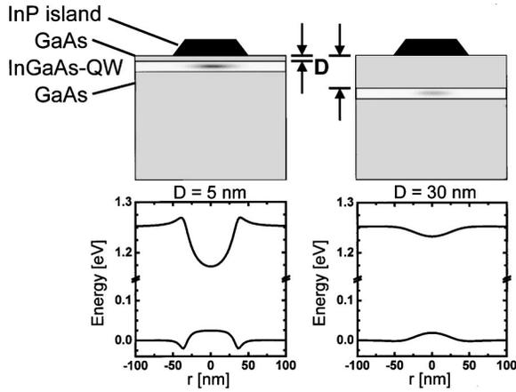
FIG. 1. Illustration of the sample design showing the effect of the thickness  $D$  of the upper GaAs spacer layer on the conduction- and valence-band profiles of the buried InGaAs quantum well. When the thickness  $D$  is small (left), the strain underneath the InP island has its strongest effect on the depth of the quantum dot potential, whereas a larger  $D$  (right) reduces the depth of the quantum dot potential.
