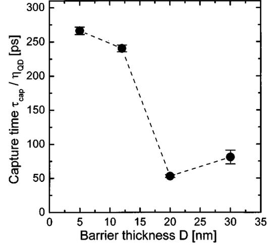
FIG. 5. Calculated quantum dot capture time  $\tau_{cap} / \eta_{QD}$  versus the GaAs spacer thickness  $D$  according to Eq. (7). The error bars reflect the uncertainties in  $I_{R,QD}$  and  $I_{R,QW}$ , as described in the text.
