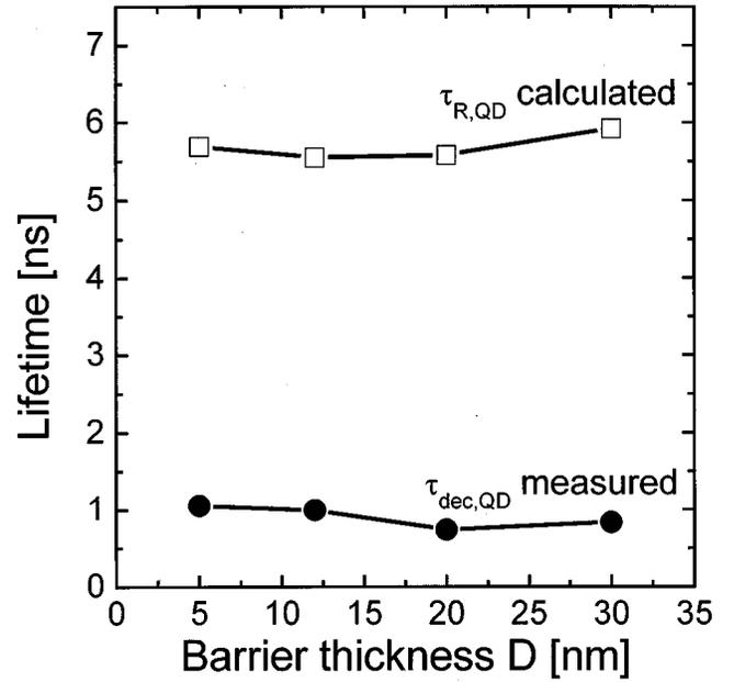
FIG. 7. Measured quantum dot ground state decay time  $\tau_{\text{dec,QD}}$  from Fig. 6 (fast-decay component) and calculated radiative decay time  $\tau_{R,\text{QD}}$  as a function of the thickness  $D$  of the top GaAs spacer layer.
