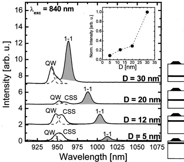
FIG. 3. Photoluminescence spectra upon nonresonant excitation in the InGaAs quantum well at 840 nm excitation wavelength for varying thickness  $D$  of the GaAs spacer layer. The quantum dot ground state transitions (1-1) are shaded. The dashed lines are Gaussian fits to resolve the QW and CSS lines. The spectra are shifted by a constant value for clarity. The inset shows the intensity of the quantum dot ground state transition as a function of  $D$ .
