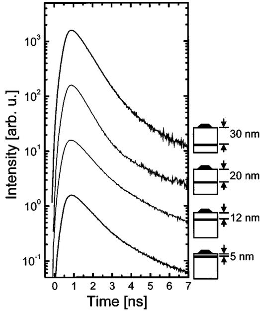
FIG. 6. Quantum dot ground state decay curves upon nonresonant excitation in the InGaAs quantum well at 840 nm excitation wavelength for varying GaAs spacer thickness  $D$ . The curves are shifted by a constant factor for clarity.
