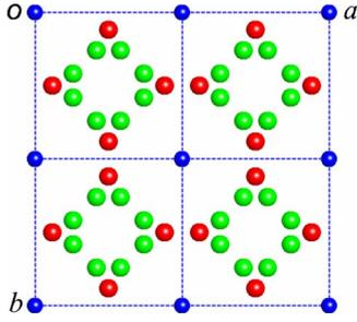
FIG. 4. (Color online) The  $(\text{Cu,Mo})\text{O}_{1+\delta}$  layer. Atomic positions for the extra oxygen atoms O5 ( $x\ y\ 0$ ; green or light shade) and O6 ( $\frac{1}{2}\ y\ 0$ ; red or dark shade) are shown. The sites are only partially occupied. Blue spheres (corners) represent Cu/Mo.
