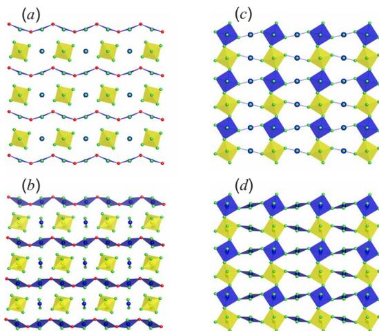
FIG. 6. (Color online) View along the [001] direction for the short-range ordered (Cu1,Mo) $O_{1+\delta}$  models (a) before and (c) after oxygenation. Tilted views are displayed in (b) and (d) to show the various Cu coordinations in the AS and HPO samples.
