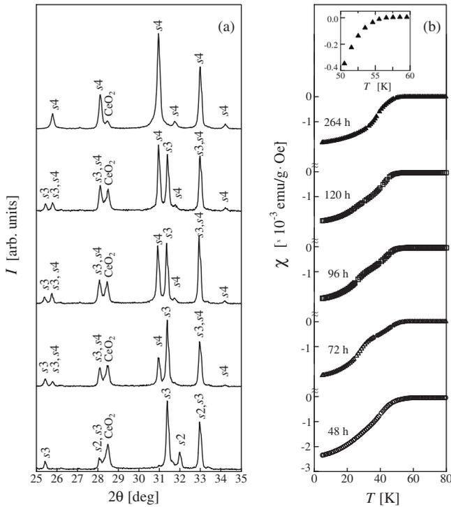
FIG. 1. (a) Evolution of the XRD patterns for the  $(\text{Cu}_{0.75}\text{Mo}_{0.25})\text{Sr}_2(\text{Ce}_{0.75}\text{Y}_{0.25})_4\text{Cu}_2\text{O}_{13+\delta}$  sample synthesized from a nitrate precursor through several repeated heat treatments in air at 950–985 °C. (b) Magnetic-susceptibility data (for the corresponding HPO samples) with consecutive heat treatments. The given heat treatment duration indicates the total accumulated time used for the consecutive heat treatments.
