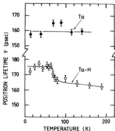
FIG. 3. Recovery of the average positron lifetime  $\bar{\tau}$  in  $\alpha$ -irradiated Ta. Hydrogen trapping at irradiation-induced vacancies is seen as a small drop of  $\bar{\tau}$  between 60–70 K in Ta-H.
