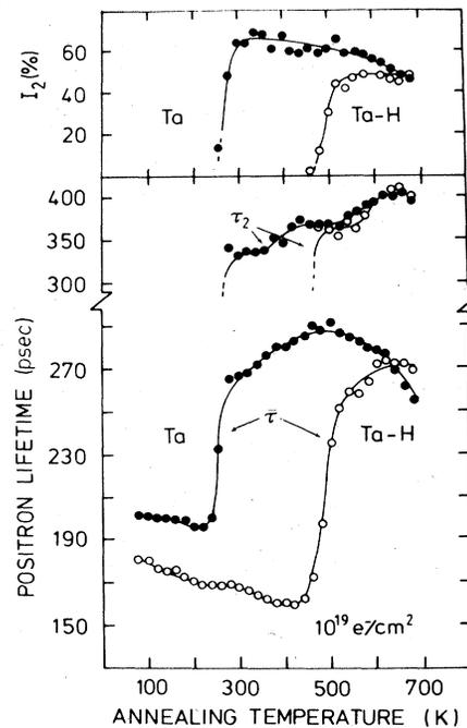
FIG. 2. Average positron lifetime  $\bar{\tau} = I_1\tau_1 + I_2\tau_2$  and the longer lifetime component  $\tau_2, I_2$  in electron-irradiated Ta as a function of annealing temperature. The increase of  $\bar{\tau}$  and the appearance of the  $\tau_2$  component shows the vacancy migration and clustering at 260 K in pure Ta. The vacancies in Ta-H are blocked by hydrogen atoms and vacancy clustering is shifted to 450 K.
