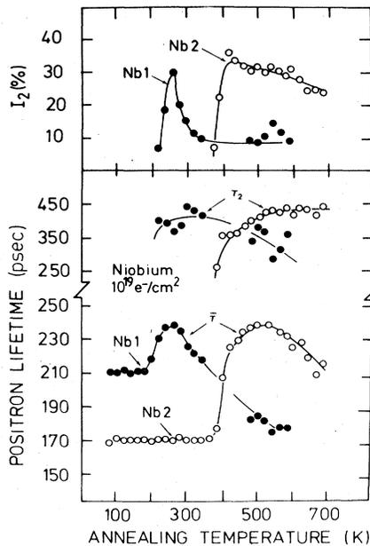
FIG. 4. Average positron lifetime  $\bar{\tau}=I_1\tau_1+I_2\tau_2$  and the longer lifetime component  $\tau_2, I_2$  in electron-irradiated Nb as a function of annealing temperature. The increase of  $\bar{\tau}$  and the appearance of the  $\tau_2$  component at 220 K in sample 1 is attributed to vacancy migration and clustering in pure Nb. In sample 2 the vacancy clustering is shifted to 380 K due to hydrogen impurities.
