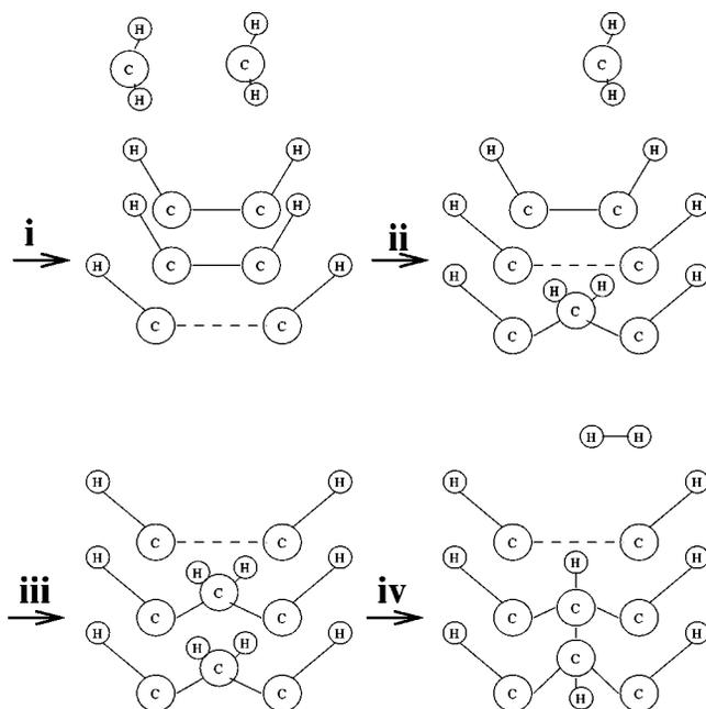
FIG. 5. Growth model with N doping of CVD (100):H diamond: the zipper mechanism. (i) The extra electron from N migrates to the surface and opens a dimer bond. (ii) A  $\text{CH}_2$  adsorbs to the open dimer and the neighboring dimer is opened. (iii) Another  $\text{CH}_2$  adsorbs to the open dimer and the next dimer is opened. (iv)  $\text{H}_2$  is abstracted and a new isolated dimer is formed to the upper terrace.
