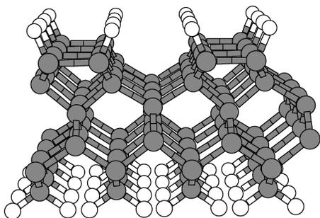
FIG. 1. Model of the reconstructed diamond (100):H(2×1) surface.
