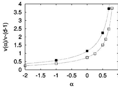
FIG. 1. Maxflow exponents measured for two-dimensional (2D) (empty squares) and 3D (filled squares) percolation clusters at  $p_c$ . Dotted lines indicate the theoretical result  $v(\alpha)/\nu - (d-1) = 1/\nu(1-\alpha)$ , with  $1/\nu=0.75$  (2D) and  $1.13$  (3D). The maximum linear size simulated was  $L=4000$  in two dimensions and  $L=120$  in three dimensions. Error bars are smaller than symbol sizes.
