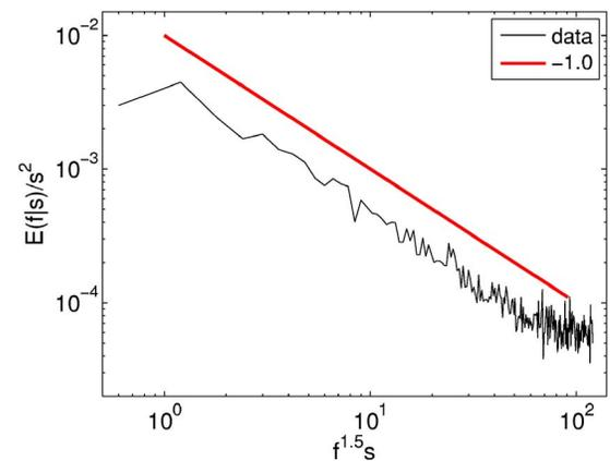
FIG. 3. (Color online) The scaled energy spectrum of dislocation avalanches, showing the form of the scaling function  $g_E(x)$ , which is consistent with the  $g_E(x) \sim 1/x$  behavior, indicated by the thick solid line. The data have been obtained by computing the energy spectrum  $E(f|s)$  of each avalanche for  $\sigma=0.03$  and  $L = 300b$ , normalizing by  $s^2$ , and averaging over all avalanches longer than a threshold duration.
