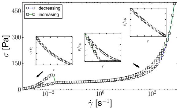
FIG. 6. (Color online) Example of a flow curve computed with the gap width  $\delta = 10$  mm and  $t_w = 160$  s. Insets: The hysteresis is more pronounced at intermediate shear rates due to the increased flow heterogeneity as shown in these velocity profiles; shear rates corresponding to the velocity profiles are  $0.001 \text{ s}^{-1}$  (left),  $100.0 \text{ s}^{-1}$  (center), and  $540 \text{ s}^{-1}$  (right).
