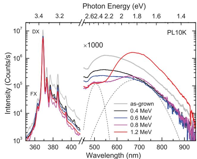
FIG. 2. (Color online) PL spectra from electron irradiated samples measured at 10 K. Note a  $\times 1000$  prefactor for the deep level related emission components. Dashed lines indicate the position and width of the observed red and green emission bands. *FX* and *DX* denote free- and donor-bound exciton recombination, respectively.
