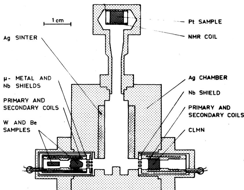
FIG. 1. Experimental cell.
