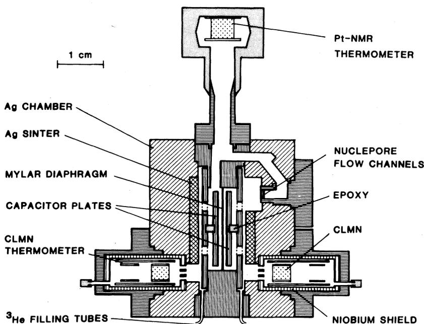
FIG. 1. Schematic diagram of the experimental cell.
