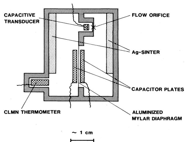
FIG. 1. Schematic illustration of our experimental  $^3\text{He}$  chambers (Ref. 9). The liquid volume  $V = 2 \text{ cm}^3$  in each compartment and the surface area of the circular diaphragm  $A = 2.7 \text{ cm}^2$ .
