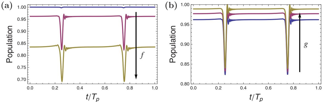
FIG. 3. (Color online) Population of the ground state of  $\tilde{H}_S+\hbar w$  in the quasistationary evolution. (a) Evolution with  $g=0.01$  and  $f=10, 75,$  and  $100$  MHz from top to bottom. (b) Evolution in presence of environmental noise for a nonadiabatic 75 MHz cycle with  $g=0.01, 0.0125,$  and  $0.015$  from bottom to top. The other parameters are the same as in Fig. 2.
