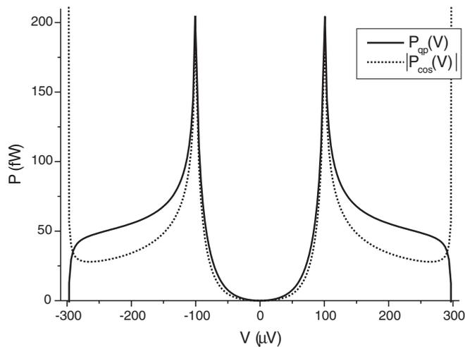
FIG. 2. The quasiparticle cooling power  $P_{qp}(V)$  (solid line) and the absolute value of the amplitude  $|P_{\cos}(V)|$  (dotted line). The parameters are chosen as follows:  $\Delta_1 = 100 \mu\text{eV}$ ,  $\Delta_2 = 200 \mu\text{eV}$ ,  $R = 1 \text{ k}\Omega$ ,  $T_1 = T_2 = 230 \text{ mK}$ .
