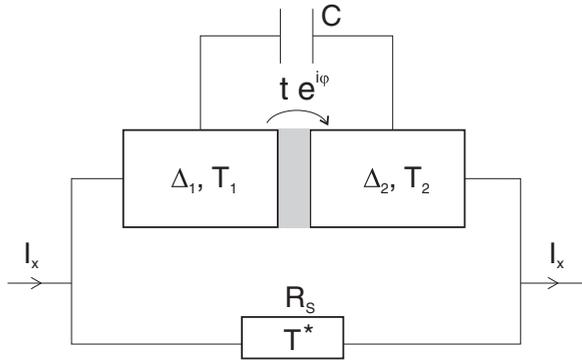
FIG. 1. A Josephson junction between two superconductors with the gaps  $\Delta_1, \Delta_2$  and temperatures  $T_1, T_2$ . The junction is shunted by a capacitor  $C$ , a resistor  $R_S$ , and the whole circuit is biased by a current  $I_x$ . The dynamics of this circuit is described by RCSJ model (7).
