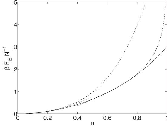
FIG. 1. Ideal free energy as a function of  $u$  in the one-mode approximation to the EOF model, as indicated in Eq. (24) with  $a_{id}=3/4$  and  $b_{id}=1/5$  (solid line). Dashed lines represent the small- and large- $u$  limits obtained from the original  $F_{id}$  in the Gaussian approximation. For comparison, the dashed-dotted line shows the curve expected from a Taylor expansion of  $F_{id}$  (i.e.,  $a_{id}=b_{id}=1$ ) which is seen to significantly overestimate  $F_{id}$ .
